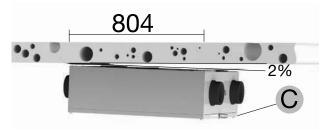
Mount the ComfoAir to a ceiling with a minimum mass of at least 200 kg/m<sup>2</sup>.
