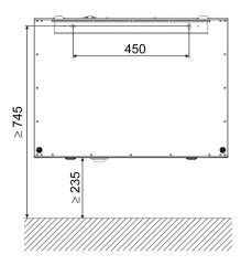
Fig. 10: FFL distance for wall mounting (version LEFT)
