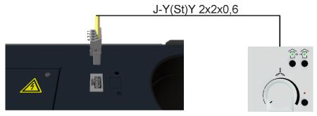
Fig. 24: Connecting cable with flat connector plug
