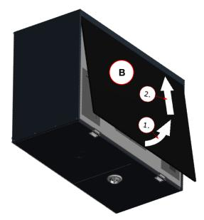
Fig. 28: Opening the front panel
