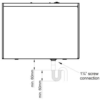
Fig. 22: Condensate drain (version LEFT)
