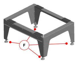
Fig. 18: Aligning the floor stand
