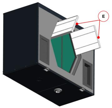
Fig. 6: Pulling out the filters
