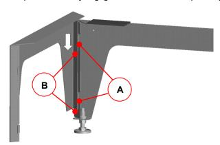
Fig. 15: Fixing the two base parts
