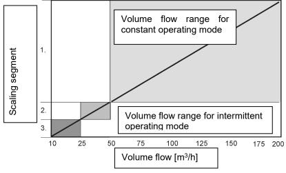
Fig. 26: Diagram 2, assignment of volume flow ranges
