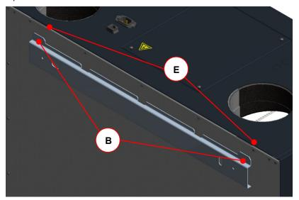
Fig. 12: Hooking the unit into the fastening sheet
