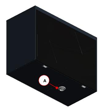
Fig. 21: Sink valve screw connection on unit version LEFT
