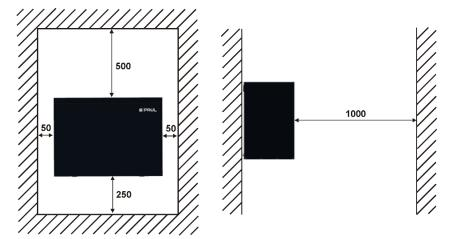
Fig. 8: Distances from adjacent surfaces in mm
