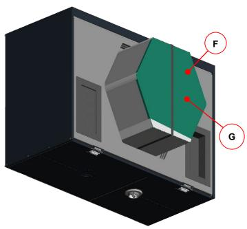
Fig. 31: Removing the heat exchanger
