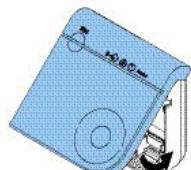
5. Replace the top section of the sensor, refitting the clips and pressing until they snap into place.
