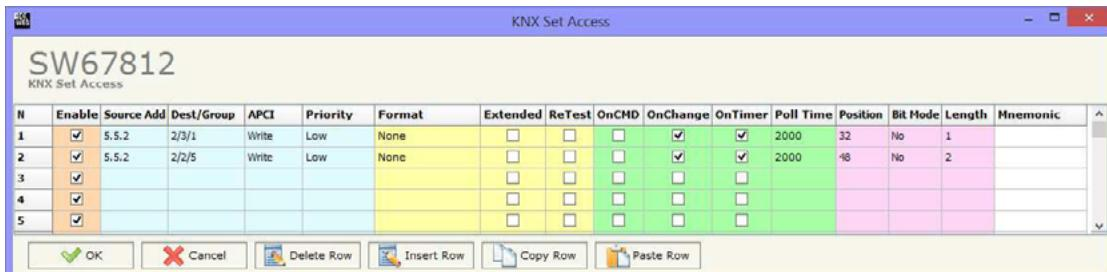
Note: If the “On Change” field is ticked and the “Poll Time” is not equal to 0, the drive sends the KNX command cyclically and also when the data is changed. If the “OnCMD”, “OnChange” and “OnTimer” fields are not ticked, the inverter only detects the bus to monitor the status of the KNX message.
