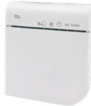
The wireless CO<sub>2</sub> sensor monitors the level of carbon dioxide in the room where it is placed and sends its readings to the Zehnder EVO unit via RF (radio frequency). The unit varies its flow rate accordingly, choosing the right level to guarantee indoor air quality on the basis of the data sent by the sensor.
