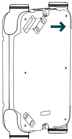
3. Gently remove the fouled filters by means of the tabs provided. If the two filters are not the same, note their positions: the ISO ePM1 filter is installed on the outdoor air inlet and the ISO Coarse filter is fitted on the room air extraction inlet.
