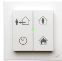
The EVO Switch 4-setting wireless push-button control device communicates with the ventilation unit via RF (radio frequency) with a choice of four different operating modes. It has a filter change alarm indicator.
