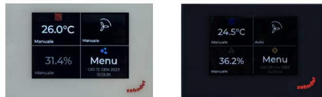
The ventilation unit takes the minimum fan speed as default. Via the relays it contains, Multi Control activates the second and third fan speeds when requested by the user or when necessary to meet post-treatment needs.
