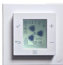
The EVO Sense wireless smart control device communicates with the ventilation unit via RF (radio frequency) and allows selection of five different flow rates. It also enables users to write daily and weekly timing programs and set automatic operating mode. It is a smart user and installation interface for supervising and configuring the connected ventilation unit.
