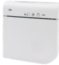
The wireless sensor monitors the relative humidity of the air in the room where it is placed and sends its readings to the Zehnder EVO unit via RF (radio frequency). The unit varies its ventilation flow rate accordingly, choosing the right level to guarantee indoor air quality on the basis of the data sent by the sensor.
